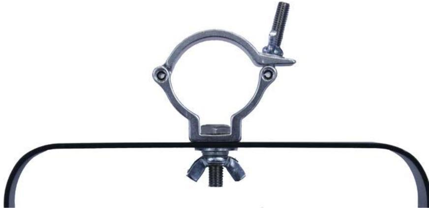
Regardless of the rigging option you choose for your MICROH SPITFIRE RGB, always be sure to secure your fixture with a safety cable. The fixture provides a built-in rigging point for a safety cable on the hanging bracket as illustrated above. Be sure to only use the designated rigging point for the safety cable and never secure a safety cable to a carrying handle.
